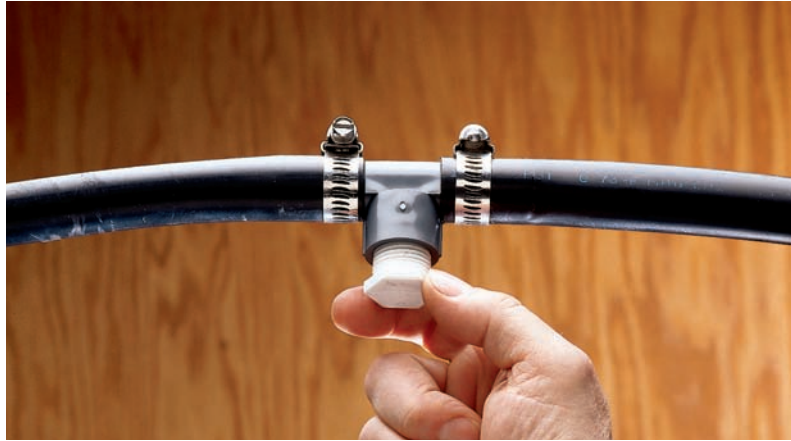
Connect lengths of PE pipe with a barbed PVC fitting. Secure the connection with stainless steel hose clamps.
